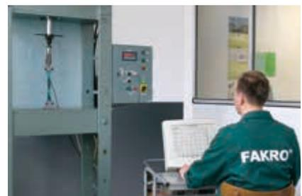
Testing resistance to tearing
