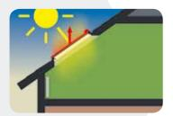
External accessories offer the best protection from high temperatures. They absorb UV radiation, protect the external glazing and keep warm air
